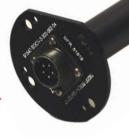
The 5000 Liquid Level Sensor utilizes stainless steel floats with highly stable magnets in conjunction with hermetically sealed reed switches. The model 5000 Liquid Level Sensor provides high-reliability low cost liquid level sensing for applications where extreme environmental conditions exist. The floats and switches are located within the structure of the sensor at specific distances to linearize the measurement of liquid based upon a mechanical model of the fluid reservoir.
