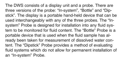
The Display is battery operated and has the storage capability for twenty different non-conductive test fluids, including fluid identification numbers. The characteristics for these or other fluids are pre-programmed into the Display memory for recall by the user.
