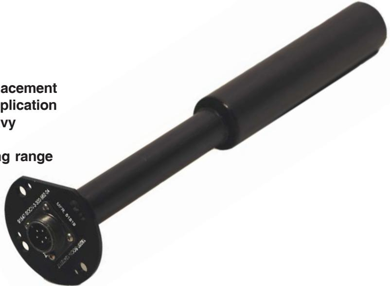
The 5000 Liquid Level Sensor utilizes stainless steel floats with highly stable magnets in conjunction with hermetically sealed reed switches. The model 5000 Liquid Level Sensor provides high-reliability low cost liquid level sensing for applications where extreme environmental conditions exist. The floats and switches are located within the structure of the sensor at specific distances to linearize the measurement of liquid based upon a mechanical model of the fluid reservoir.
