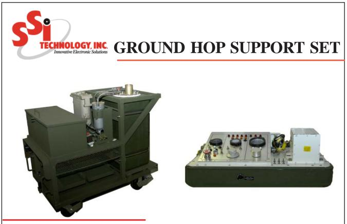
The GHSS is a diagnostic system that is used for fault detection and fault isolation of the M1A1 tank engine and transmission systems. The fuel cart assembly contains the fuel and delivery system to operate the M1A1 turbine engine and transmission while it is in the M1 Tank. The Control Panel is used to start, operate and perform diagnostic tests on the entire FUPP.
